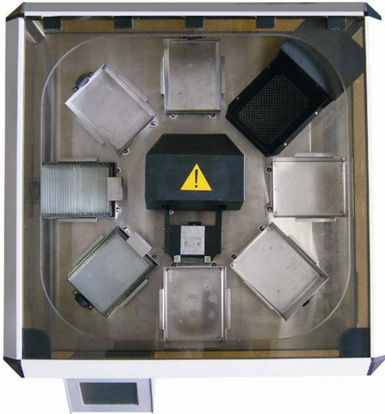
Fig. 2 Working chamber of the automatic slide stainer AFOMK8-G-01 (cover is open, it is not shown) with the installed vessels, trays and holders. The manipulator used to move holders is shown in the center of the picture.
